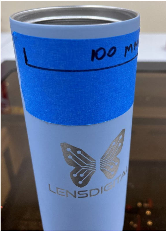
Figure 17: Apply tape to the tumbler
